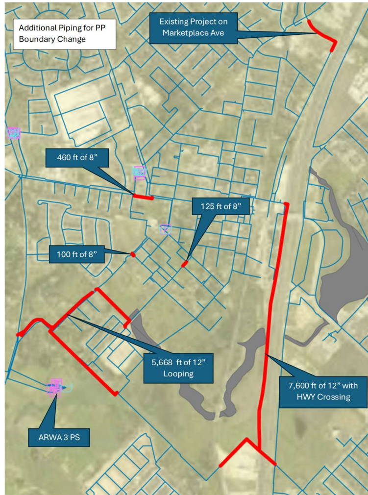
Figure 4-6 Improvements Detail for Pressure Plane Modification
