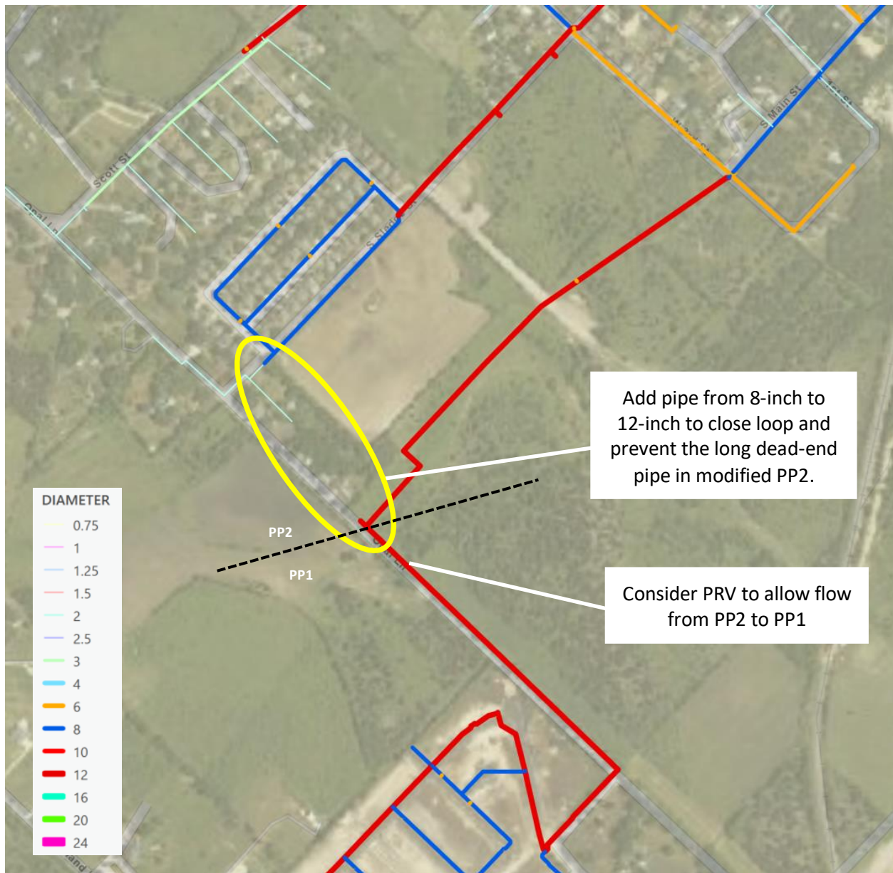
Figure 18 - Recommended New Connections within Modified Pressure Plane 2 (Part 2)
